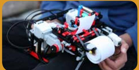
Shubham Banerjee built the prototype for the Braille printer from Lego's Mindstorms EV3 robotics kit.
